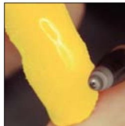
A coarse acrylic bur works well for shaping and refining a periphery.
